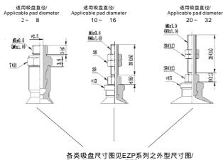
各类吸盘尺寸图见EZP系列之外型尺寸图/ Pad dimension as EZP outline drawing
