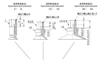
各类吸盘尺寸图见EZP系列之外型尺寸图/ Pad dimension as EZP outline drawing
